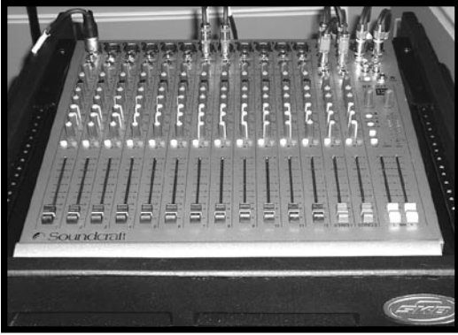
This is a Soundcraft Spirit E12, 12-channel mixer. Larger ensembles may need a 16-channel mixer.
